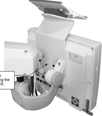
**4.** Mount ventilator display on Mounting Bracket by hanging the four (4) SHCS in the keyholes. Using the 3mm hex wrench provided, tighten four (4) SHCS.
