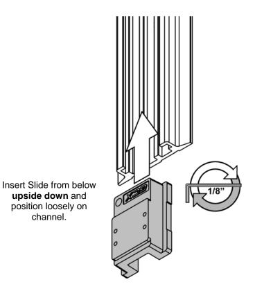
2. Install the CPU mount with attached with bottom Channel Slide attached and secure to the desired height using the 1/8" hex wrench provided.
