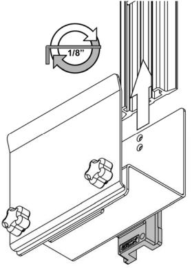
Insert lower Slide to the desired height and tighten using 1/8" hex wrench. 3. Move the top Slide in positon to align with CPU Mount holes. Using a Philips screwdriver, tighten the four #10 x 3/4" FHMS. Finally using the 1/8" Hex Wrench provided, tighten the Set Screw for the upper Slide.
