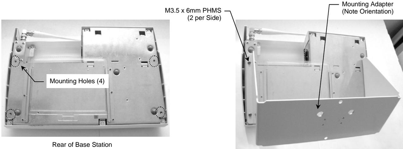
3. Slide the Adapter onto the Mounting Plate until the Adapter makes contact with the Plunger. Pull the Plunger downward and hold in position while sliding the Adapter over the Plunger. Release Plunger and continue sliding the Adapter until the Plunger snaps into the clearance hole.
